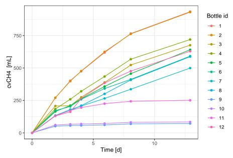
Plotting results is recommended, and can be used to catch strange responses like for bottle # 2 here.
